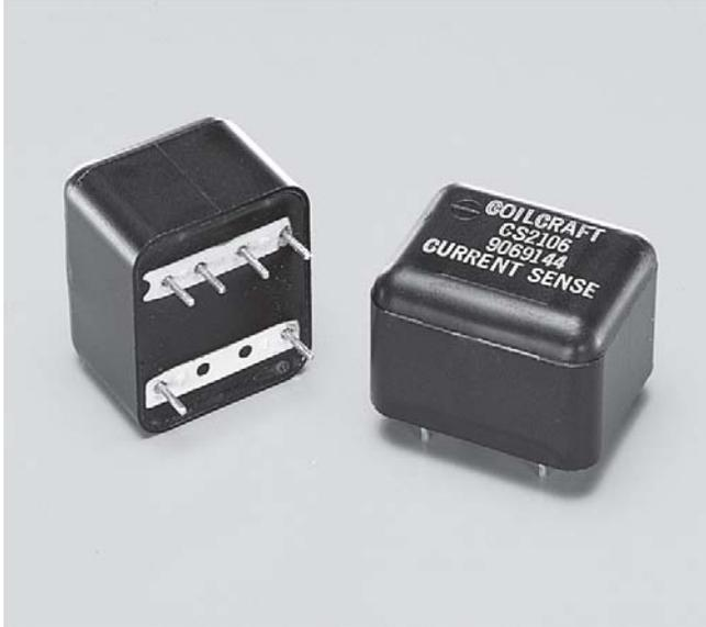
This Coilcraft current sense transformer is intended for use in measuring 50/60 Hz line currents from 0.5 to 20 Amperes rms. Typical application shown below yields an output of 0.1 Volt per Ampere. The sensitivity may be changed by adjusting the value of the terminating resistance ( $R_T$ ). These parts also can be used to measure 400 Hz line currents.
