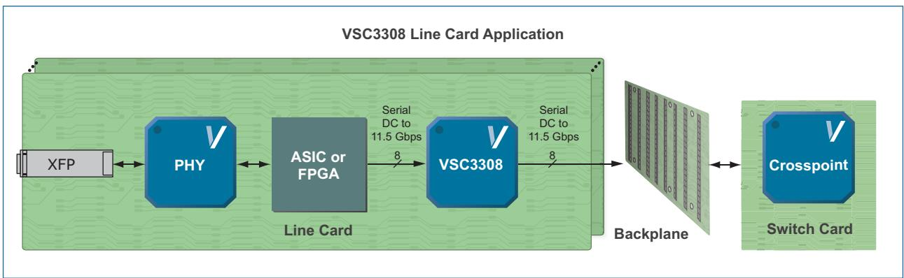
Using the VSC3308 in high-speed line cards ensures best-in-class I/O performance up to 11.5 Gbps with EQ technology to compensate for connector, backplane, and FR-4 loss.
