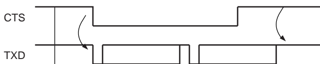
Figure 38-28. Transmitter Behavior when Operating with Hardware Handshaking
