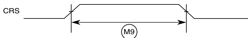
Figure 43. MII async inputs timing diagram
