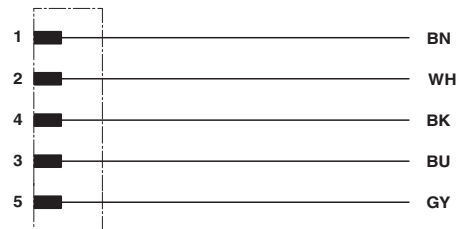
Contact assignment of the M12 plug
