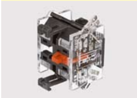
Switching element, plug-in terminal, 6.3 mm, slow-make with forced opening silver contacts
