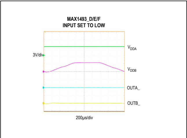
Figure 5. Undervoltage Lockout Behavior (MAX1493_ D/E/F Low)
