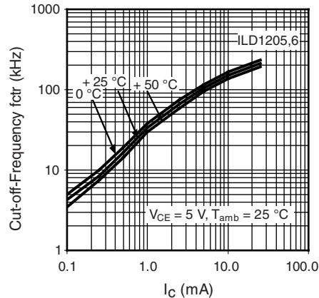
Figure 8. Cut-off-Frequency (- 3 dB) vs. Collector Current
