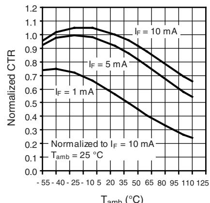
Normalized CTR vs. Ambient Temperature
