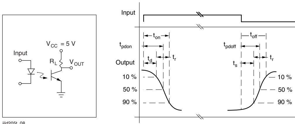
Figure 2. Switching Test Circuit
