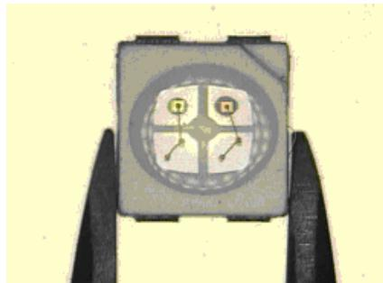
3) When populating boards in SMT production, there are basically no restrictions regarding the form of the pick and place nozzle, except that mechanical pressure on the surface of the resin must be prevented. This is assured by choosing a pick and place nozzle which is larger than the LED's reflector area.
