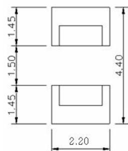
( Tolerance:  $\pm 0.2$ , Unit: mm )
