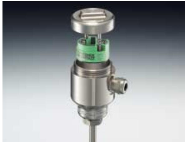
**Universal PC programmable temperature measuring transducers** convert temperature signals from resistance thermometers and thermocouples as well as sensors with linear mV characteristic curves to analog 4...20 mA signals.
