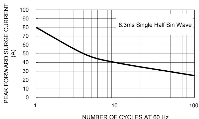
FIG. 2 MAXIMUM FORWARD SURGE CURRENT
