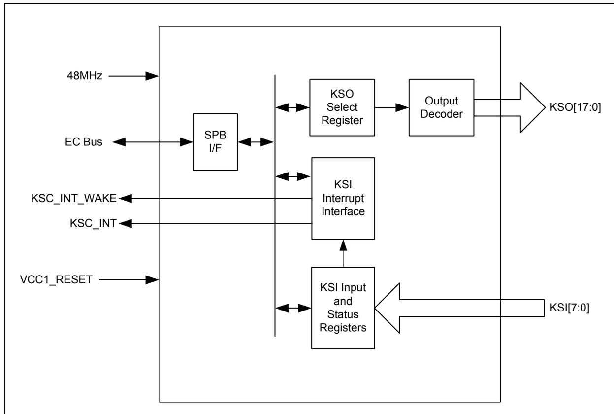
During scanning the firmware sequentially drives low one of the rows (KSO[17:0]) and then reads the column data line (KSI[7:0]). A key press is detected as a zero in the corresponding position in the matrix. Keys that are pressed are debounced by firmware. Once confirmed, the corresponding keycode is loaded into host data read buffer in the 8042 Host Interface module. Firmware may need to buffer keycodes in memory in case this interface is stalled or the host requests a Resend.
