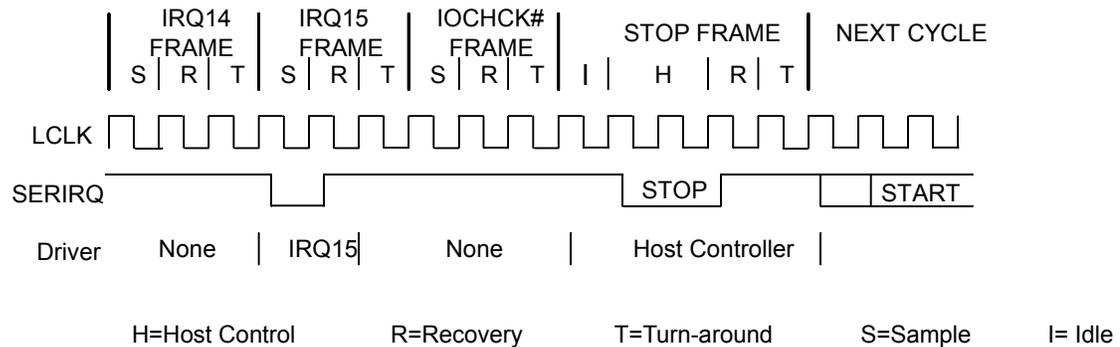
Stop pulse is two clocks wide for Quiet mode, three clocks wide for Continuous mode.
