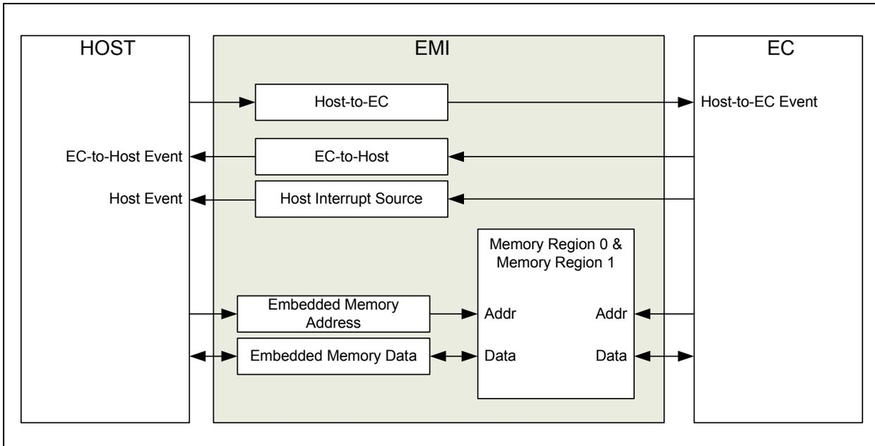
The Embedded Memory Interface (EMI) is composed of a mailbox, a direct memory interface, and an Application ID register.
