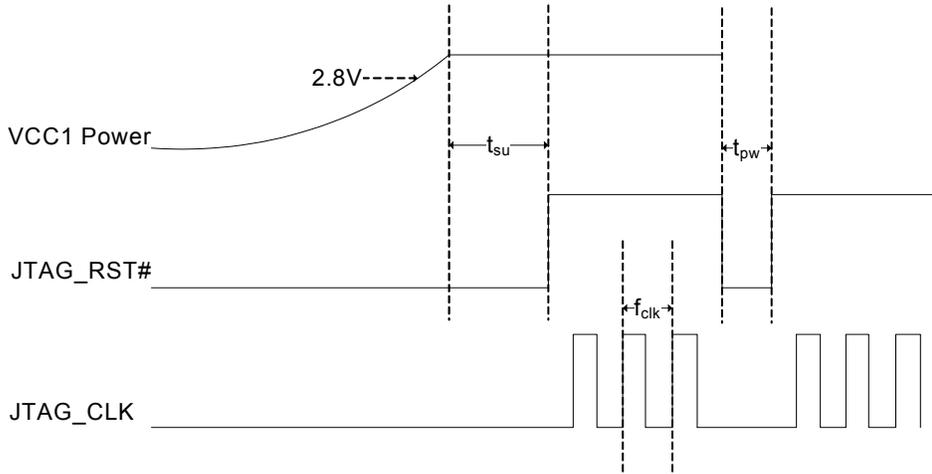
FIGURE 38-33: JTAG SETUP & HOLD PARAMETERS
