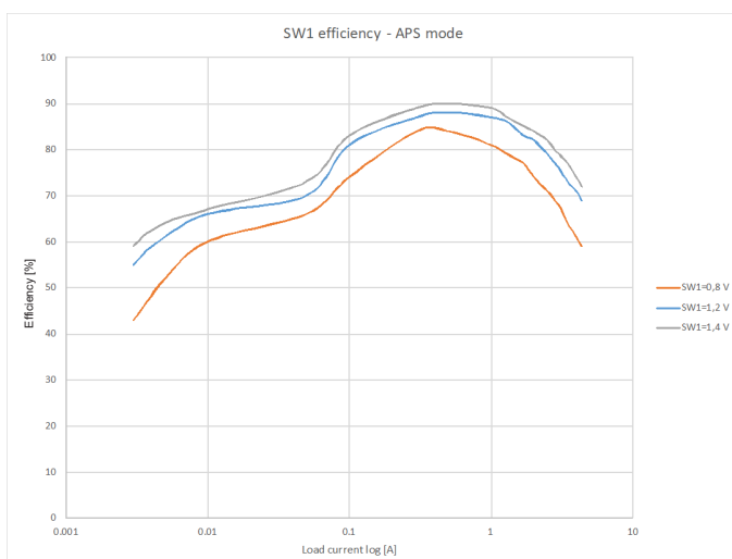
Figure 25. SW1 efficiency - APS mode
