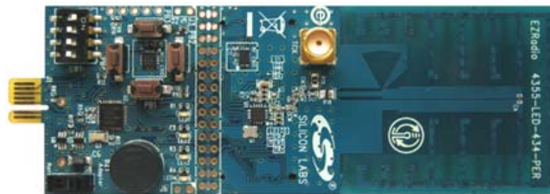
Figure 2. Si4355 RFStick 434 MHz Receiver Board (P/N 4355-LED-434-SRX)
