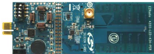
Figure 2. Si4355 RFStick 434 MHz Receiver Board (P/N 4355-LED-434-SRX)
