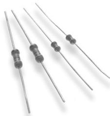
The LT temperature sensing resistors are trimmed to specification on latest equipment. The case construction epoxy coated with axial leads, permits automatic insertion with available tape and reel packaging.
