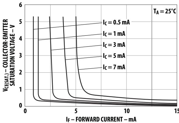
Figure 3. Collector-emitter saturation voltage vs. forward current.
