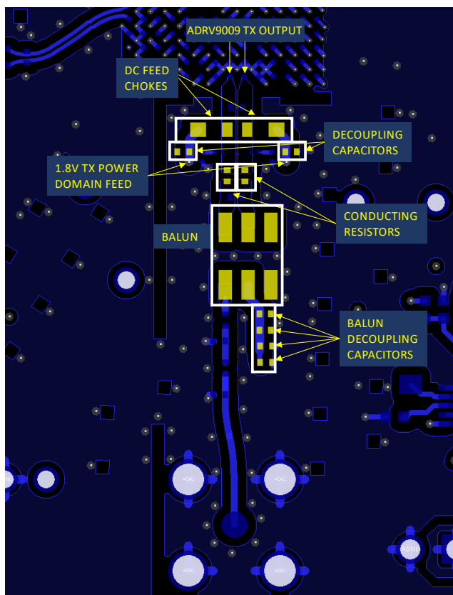
Figure 443. Transmitter DC Chokes and Balun Feed Supply
