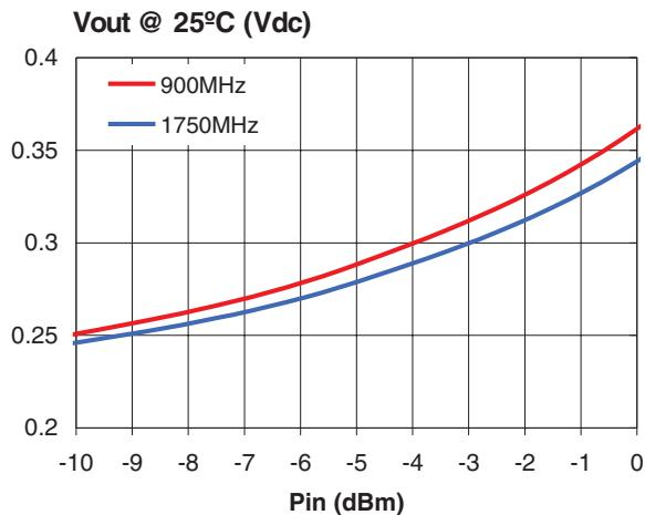
**Fig. 8:** Power detector sensitivity at low RF power.
