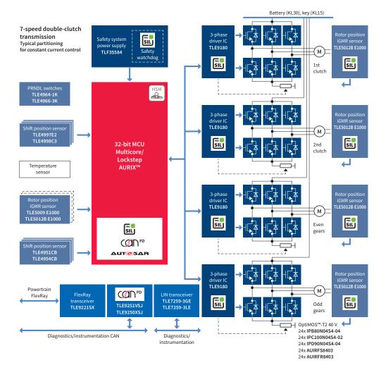
Thanks to its state-of-the-art safety features, the new TriCore™ AURIX™ family enables systems to achieve the highest safety level up to ASIL-D. The rich scalability of the AURIX™ family permits a platform approach that meets the needs of a range of transmission systems. Furthermore, the hot temperature package and bare die solutions enable AURIX™ to be used in both attached and integrated control units.
