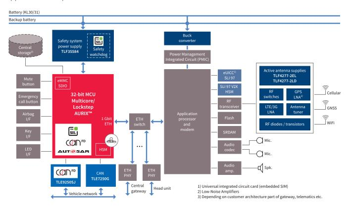
The telematics control unit connects the car to the outside world, thereby enabling numerous new applications and functionalities. Software in different ECUs can be updated remotely, to either add new features or remove any software bugs that might be found during operation. This reduces the number of recalls and related costs, while increasing customer satisfaction. The opportunity to add new features opens up the door to new business models and revenue streams.
