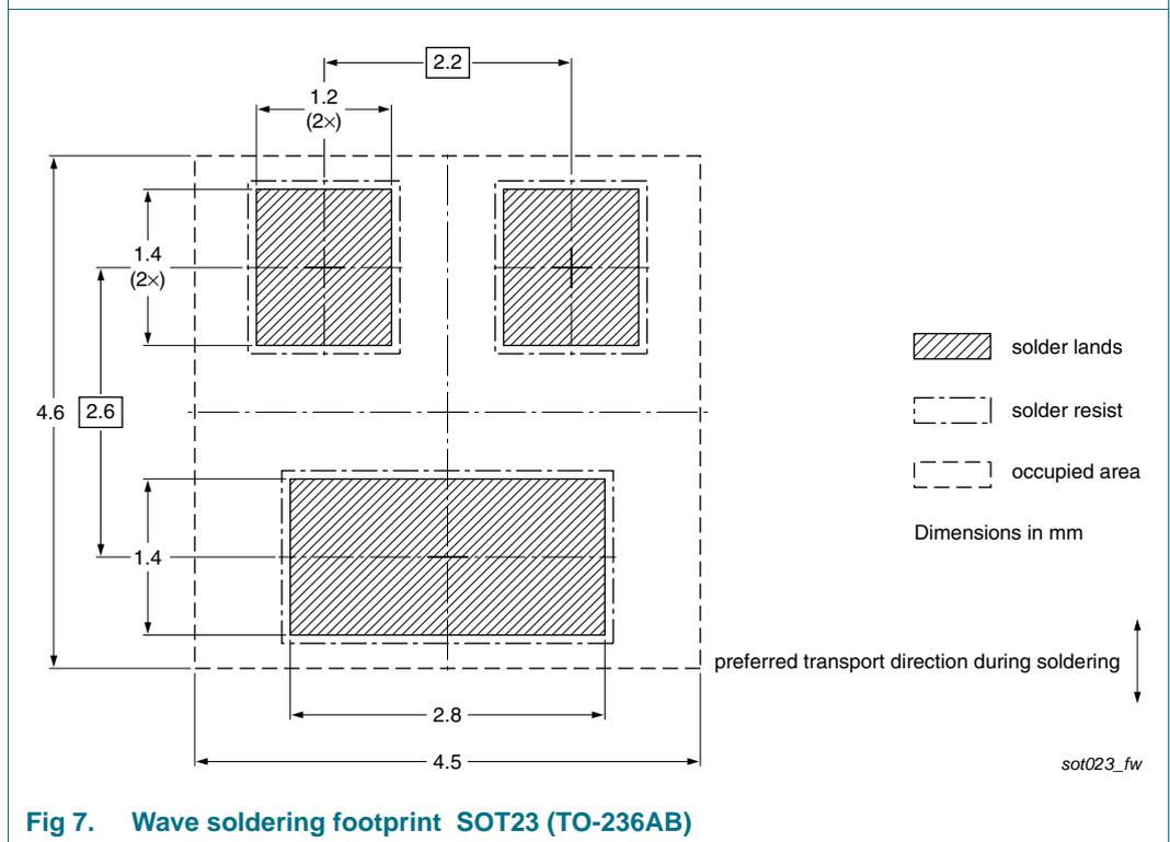
Fig 7. Wave soldering footprint SOT23 (TO-236AB)
