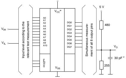
v: In measurement of  $t_{dis}$ -times and  $t_{en}$ -times the capacitance is 5 pF.
