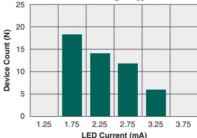
**Typical  $I_F$  for Switch Dropout
