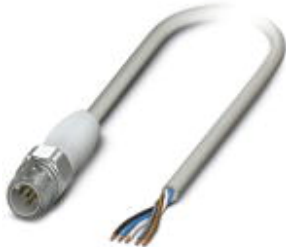
Sensor/Actuator cable, 5-position, PP-EPDM halogen-free, Gray RAL 7035, Plug straight M12, A-coded, on Free cable end, Cable length: 10 m, Hygienic design, With high-grade steel knurl
