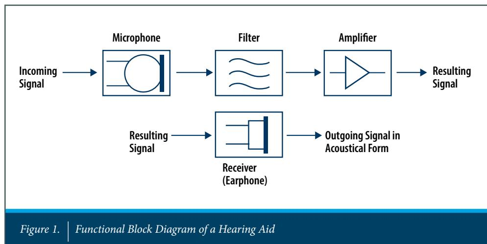
Figure 1. | Functional Block Diagram of a Hearing Aid
