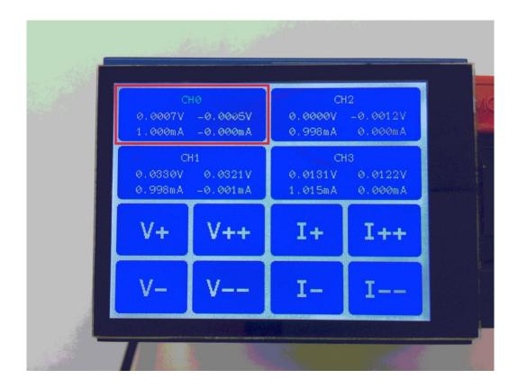
The V+, V++, V-, V--, I+, I++, I-, and I-- buttons adjust the output voltage and current of the selected channel.
