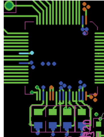
Figure 59. Top Layer Decoupling REFIN/REFOUT, REFCAPA, REFCAPB, and REGCAP Pins
