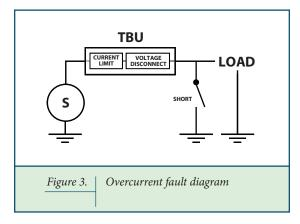
A short circuit event occurring at time 1 (see Figure 4), raises the current to the current limiting level of  $I_{out}$  time 2 (~10 nanoseconds). At this point, the voltage disconnect portion of the circuit operates and by time 3 (~1 microsecond), the load is disconnected from the surge. During the remainder of the surge (time 4), the TBU device remains in the protected state of very low current and voltage at the load.
