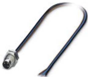
Sensor/actuator flush-type plug, 3-pos., M8, rear/screw mounting, with M8 thread, with 0.5 m TPE litz wire, 4 x 0.25 mm²
