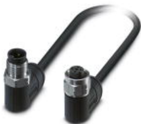
Sensor/actuator cable, 4-position, PE-X halogen-free, black-gray RAL 7021, Plug angled M12, A-coded, on Socket angled M12, A-coded, cable length: 6 m, for outdoor applications, with high-grade steel knurl
