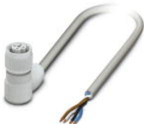
Sensor/Actuator cable, 4-position, PP-EPDM halogen-free, Gray RAL 7035, Free cable end, on Socket angled M12, A-coded, with 3 LEDs, Cable length: 3 m, Hygienic design, with plastic knurl
