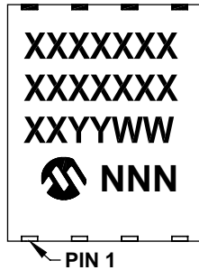
8-Lead DFN-S (6x5x0.9 mm)
