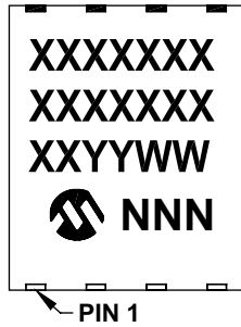
8-Lead DFN-S (6x5x0.9 mm)
