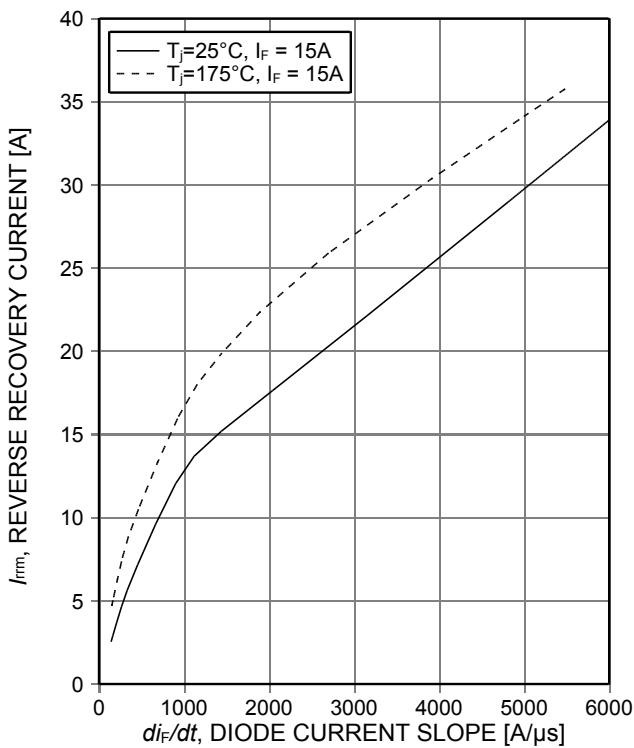
Figure 5. Typical peak reverse recovery current as a function of diode current slope ( $V_R=400\text{V}$ )
