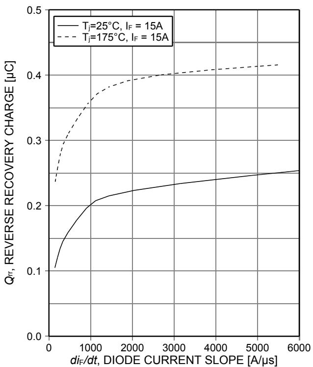
Figure 4. Typical reverse recovery charge as a function of diode current slope
