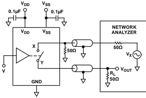
$$\text{OFF ISOLATION} = 20 \log \frac{V_{\text{OUT}}}{V_{\text{S}}}$$
