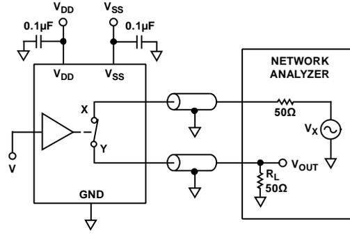
$$\text{INSERTION LOSS} = 20 \log \frac{V_{\text{OUT WITH SWITCH}}}{V_{\text{OUT WITHOUT SWITCH}}}$$
