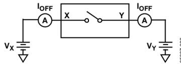
Figure 26. Off Leakage
