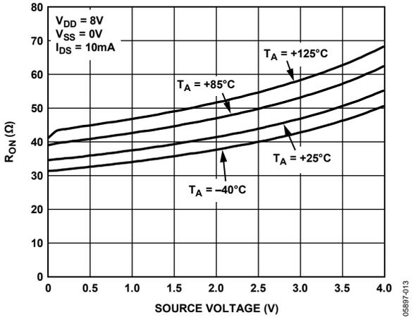
Figure 10.  $R_{ON}$  vs. Temperature,  $V_{DD} = 8\text{ V}$
