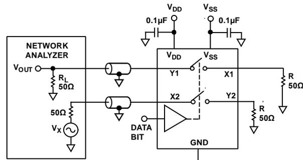
$$\text{CHANNEL-TO-CHANNEL CROSSTALK} = 20 \log \frac{V_{\text{OUT}}}{V_{\text{S}}}$$
