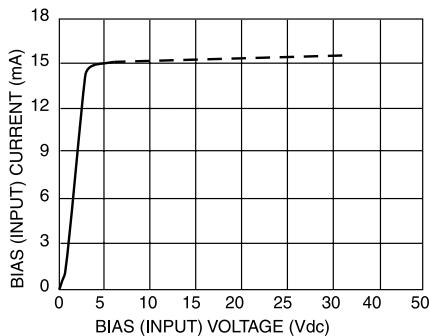
**INPUT CURRENT VS INPUT VOLTAGE FIGURE 2
