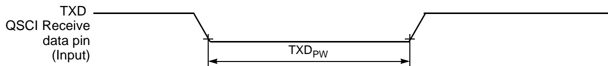
Figure 10-13 TXD Pulse Width
