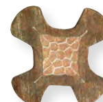
Indenter Crimp Cross-Section Across Axis
