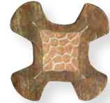
Indenter Crimp Cross-Section Across Axis
