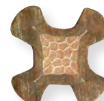
Indenter Crimp Cross-Section Across Axis
