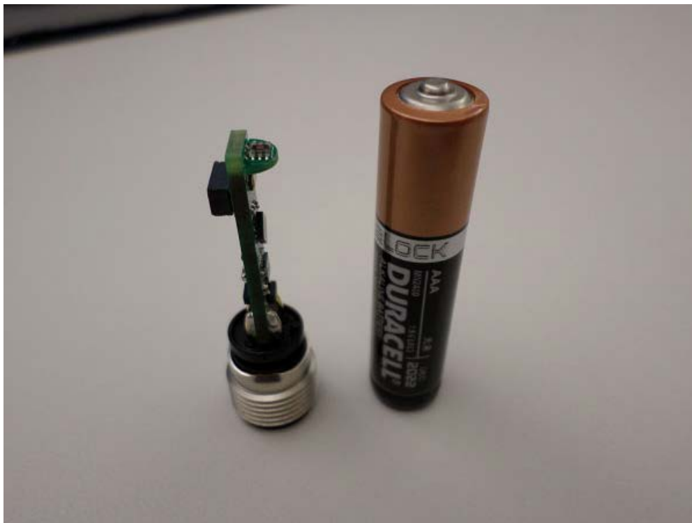
Figure 2. The Santa Cruz reference design next to a standard AAA battery.
