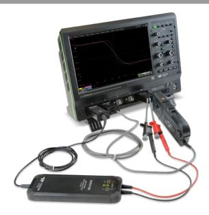
CP150 150A current probe and HVD3106 high voltage differential probe connected to an HD06104A-MS 12-bit resolution high definition oscilloscope. The DCS025 is connected to the EXT input (to conserve analog channels) and the deskew amount is adjusted for one of the probes in the channel dialog menu. In this case, a vertical Zoom of the current signal is used for deskewing.
