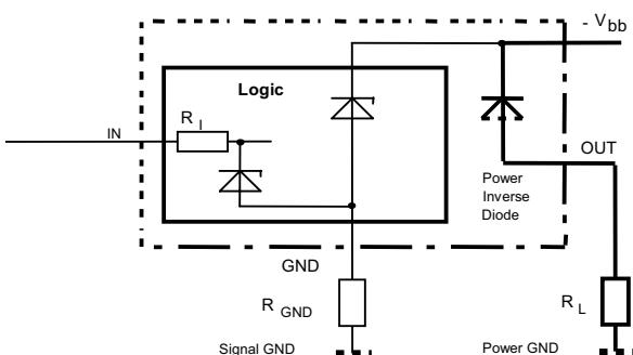
$R_{GND}=150\Omega$ ,  $R_I=3.5\text{k}\Omega \text{ typ.}$ ,
