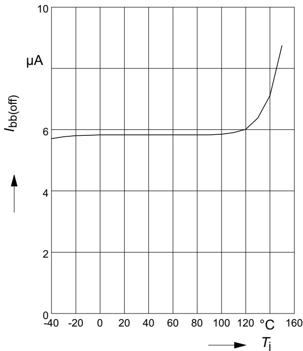
**Typ. leakage current**
