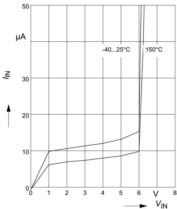
**Typ. input threshold voltage**
