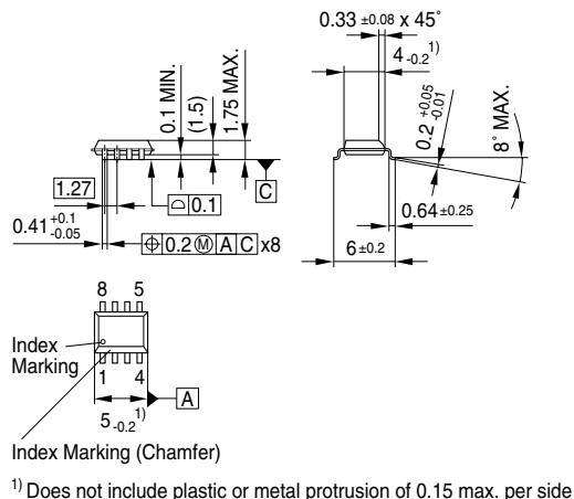
**Figure 1 PG-DSO-8-24 (Plastic Dual Small Outline Package) (RoHS-compliant)**
