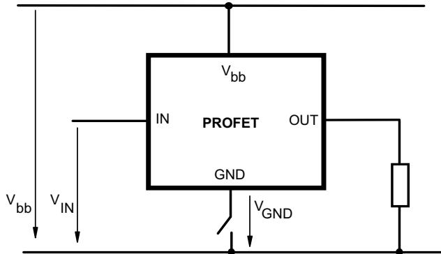
**V<sub>bb</sub> disconnect with charged inductive load**
