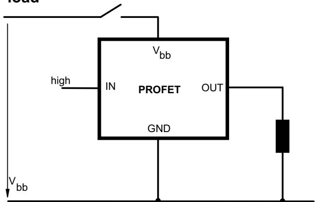
**GND disconnect with GND pull up**
