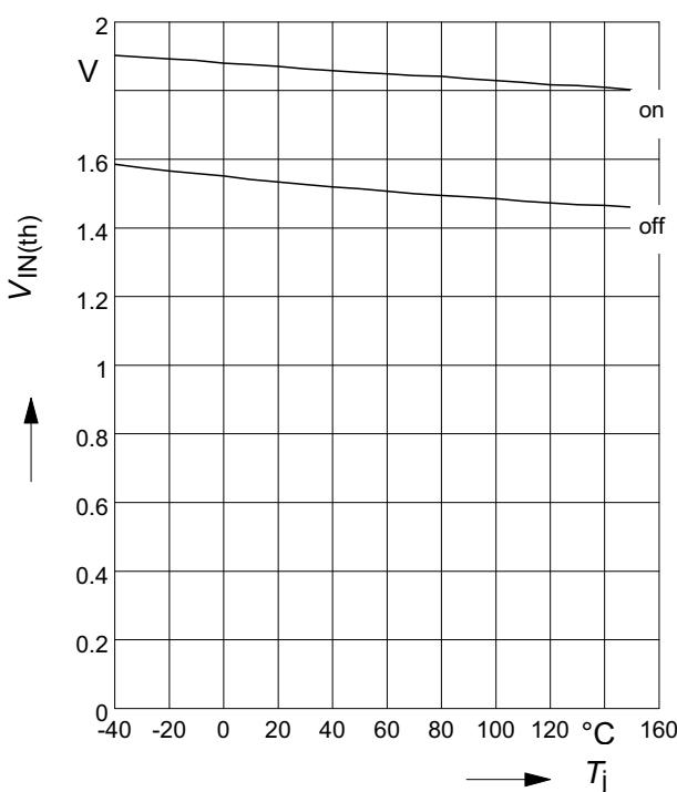
**Typ. input threshold voltage**
