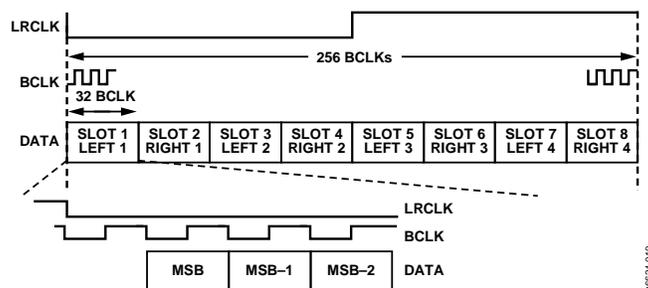
Figure 10. DAC TDM (8-Channel I<sup>2</sup>S Mode)
