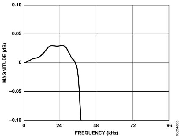
Figure 5. DAC Pass-Band Filter Response, 96 kHz
