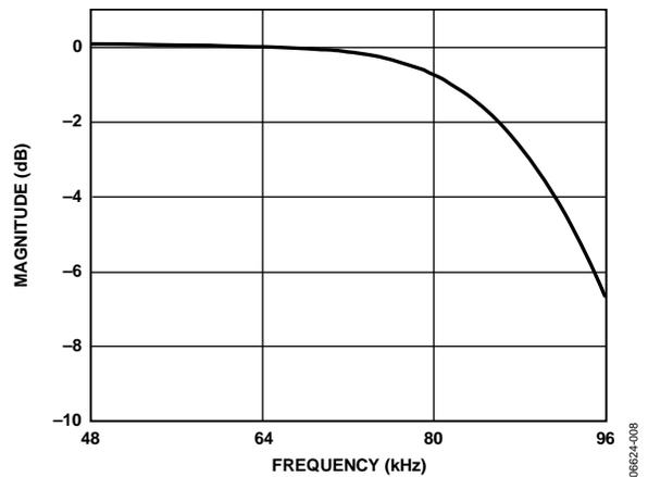
Figure 8. DAC Stop-Band Filter Response, 192 kHz
