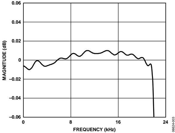
Figure 3. DAC Pass-Band Filter Response, 48 kHz
