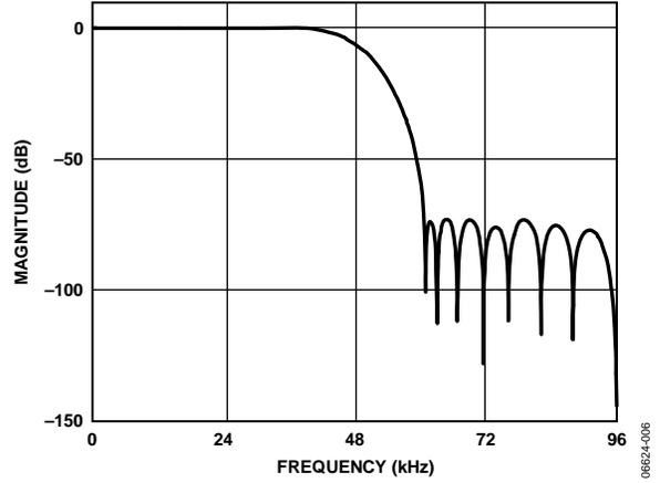
Figure 6. DAC Stop-Band Filter Response, 96 kHz
