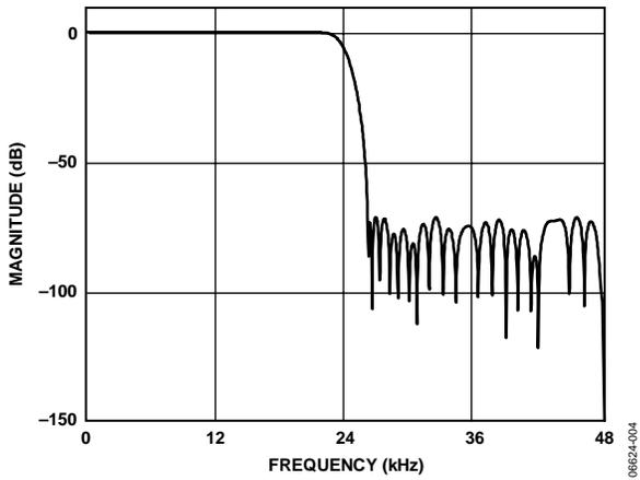
Figure 4. DAC Stop-Band Filter Response, 48 kHz
