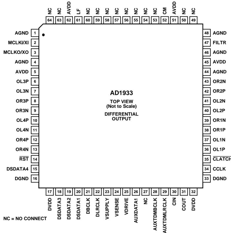
Figure 2. Pin Configuration
