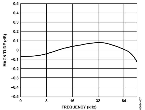
Figure 7. DAC Pass-Band Filter Response, 192 kHz
