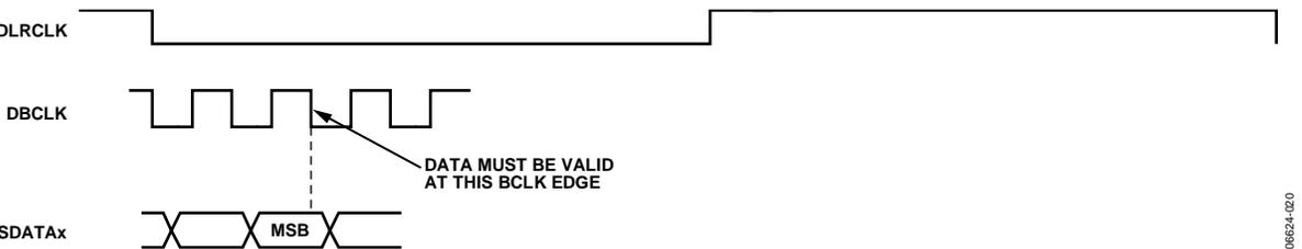
Figure 20. <sup>PS</sup> Pipeline Mode in DAC Serial Data Transmission (Applicable in Stereo and TDM Useful for High Frequency TDM Transmission)
