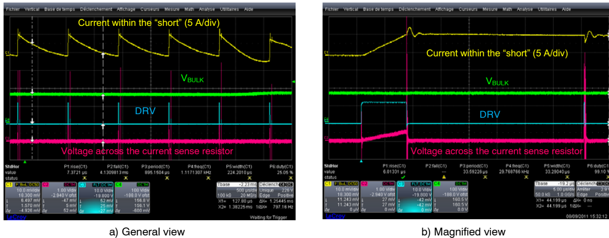
Figure 17. Shorting the Bypass Diode and the NTC
