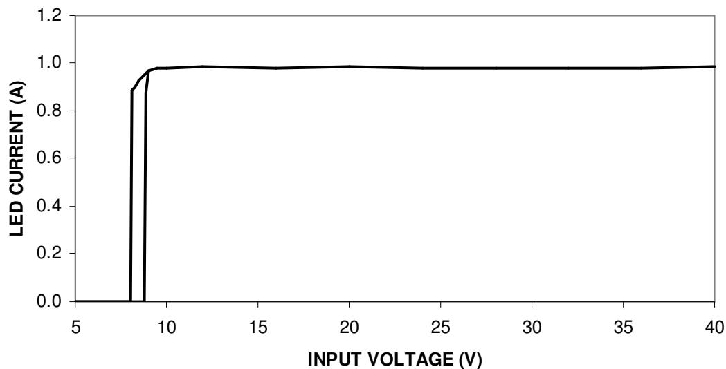
Figure 3. DC1268B-A/B LED Current Drops at Low VIN (CTRL) and Turns Off at Lower VIN (UVLO)
