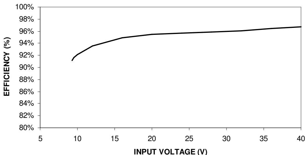
Figure 2. DC1268B-A/B Efficiency with 50V LEDs at 1A
