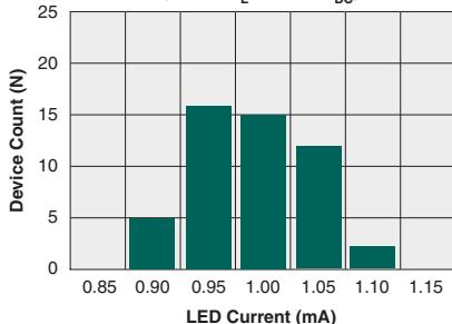
**Typical  $I_F$  for Switch Dropout
