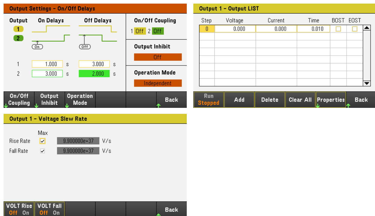
Figure 8. Output sequencing and output LIST mode, with slew rate setting
