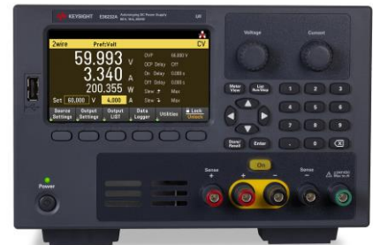
E36232A 200W Autoranging power supply 60V, 10A
