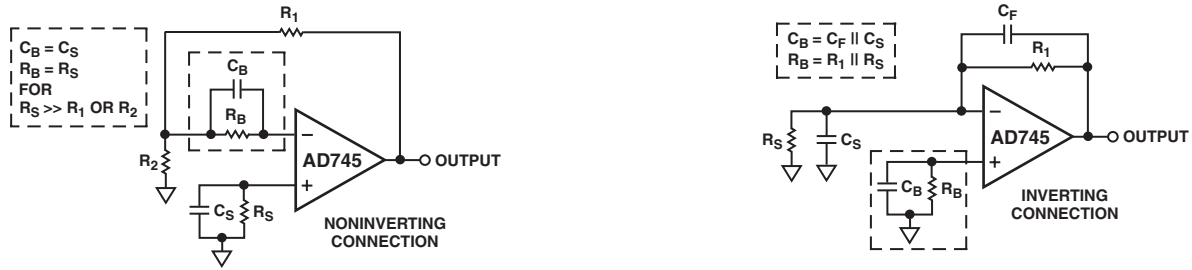
Figure 40. Optional External Components for Balancing Source Impedances
